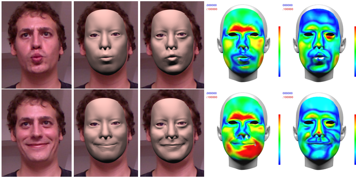
Figure 7.4: Examples of point cloud fitting error compared to ground truth. From left to right: input image, reconstruction with base multi-linear models, reconstruction with the generated blendshapes, point cloud fitting error with base multi-linear models, point cloud fitting error with the generated blendshapes. The error bar has a range of [0, 10mm]. The input images are reprinted from the FaceWarehouse dataset[35].
