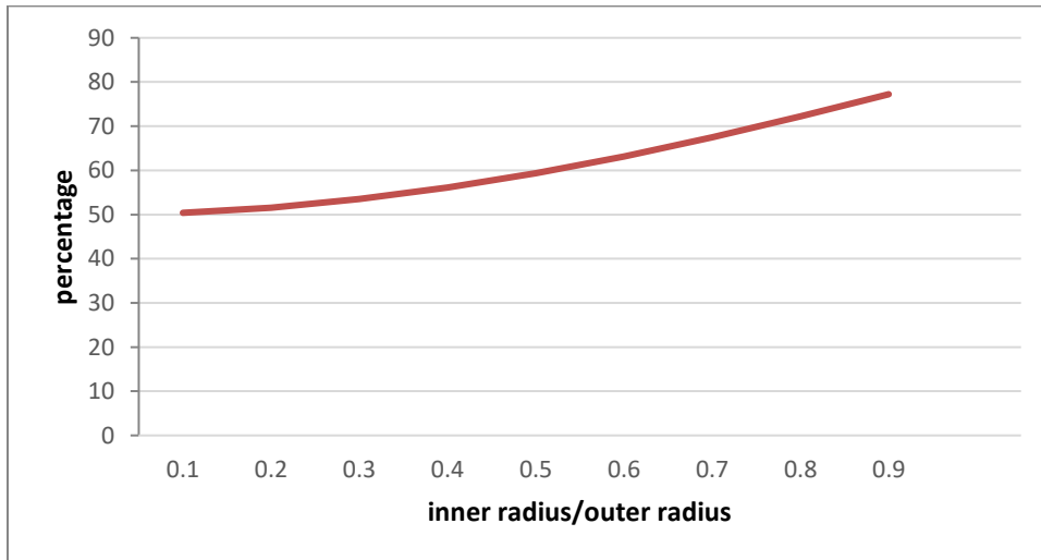
Figure 4.5 Comparison of Specific Energy: Shell vs. Shaftless Flywheel
