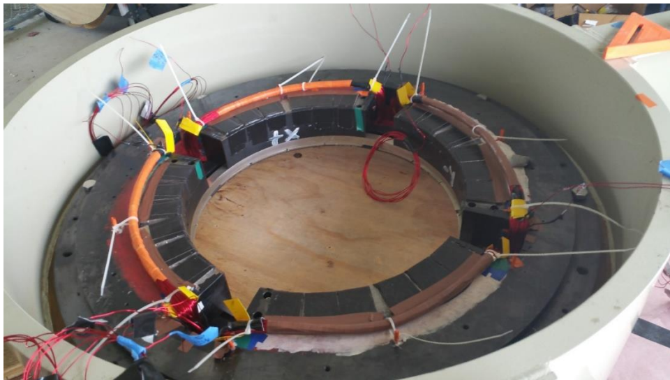
Figure 7.5 Installation of the Tilting Coils
