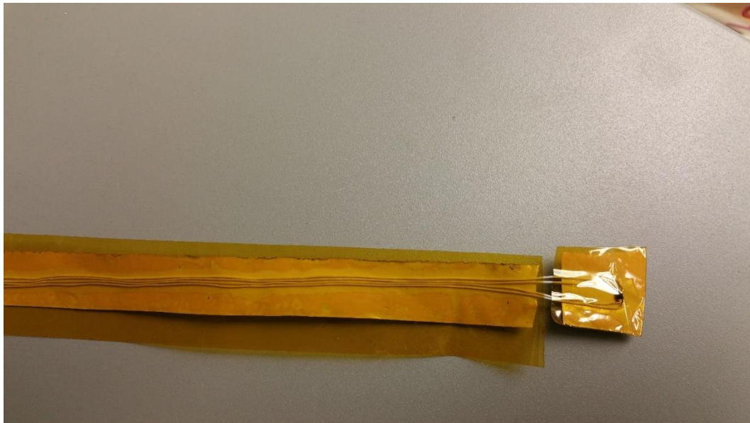
Figure 5.16 In-house Magnetic Field Density Measurement Tool
