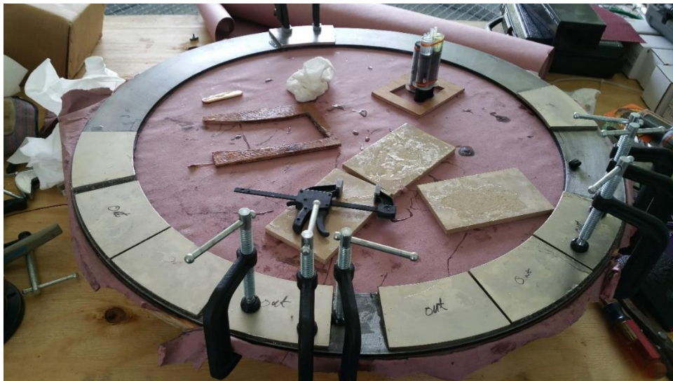
Figure 7.7 Installation of the Bottom Permanent Magnets
