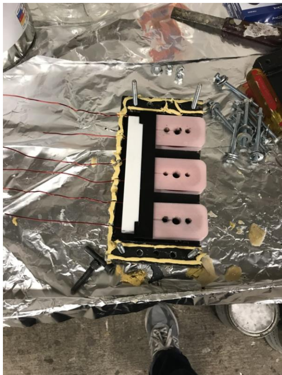
Figure 7.23 The Potting Assembly Includes Three Coils, One for Each Phase.
