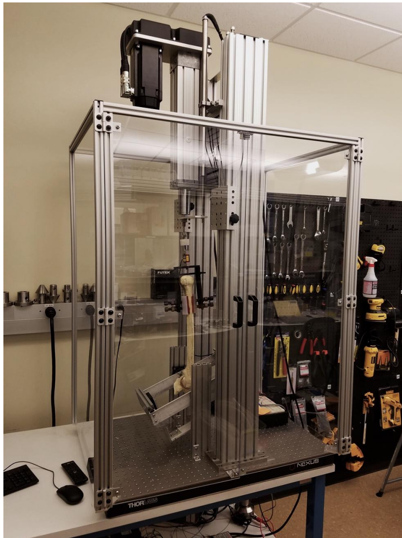
Figure 31 – The constructed RTS in a uniaxial configuration with safety screen and fixturing with a Sawbone model for an ongoing study in the BMEL to evaluate acetabular capsule repairs
