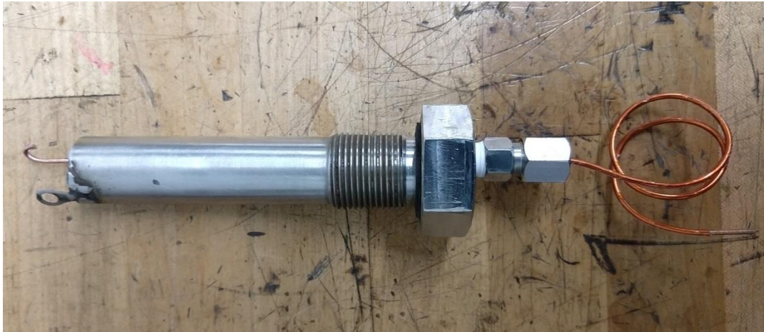
Figure 18 Bolt used to hold the propellant sample for testing
