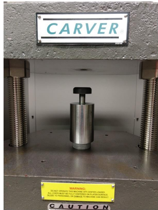
Figure 15 Pellet punch loaded between the platens of the press
