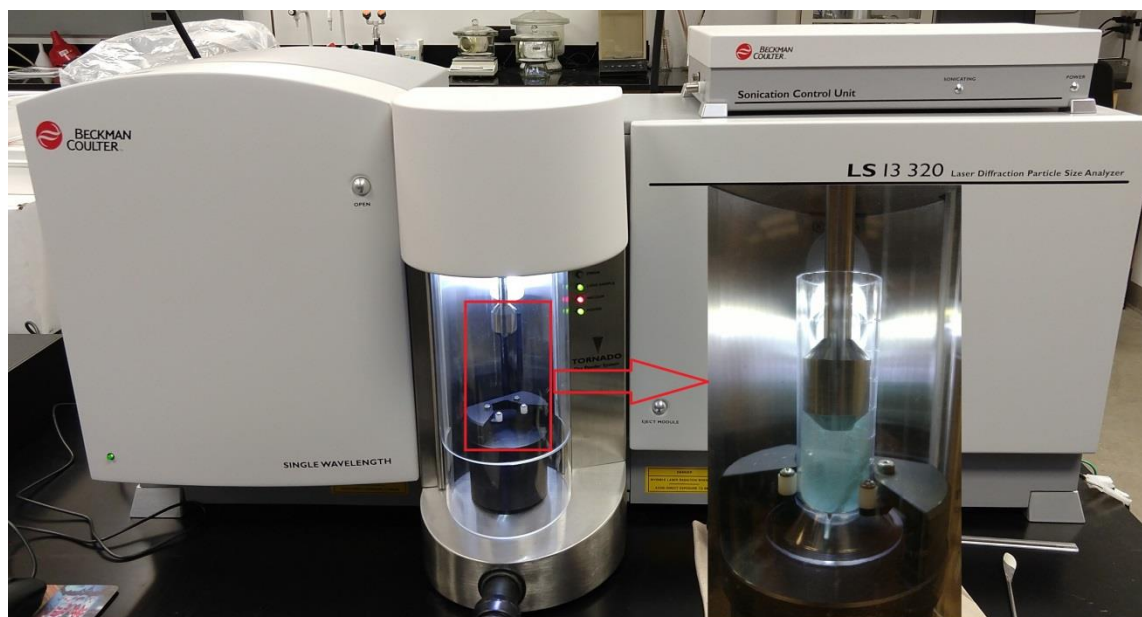
Figure 6 Laser diffraction particle size analyzer and BCN sample testing courtesy of Dr. Chad Mashuga's research group
