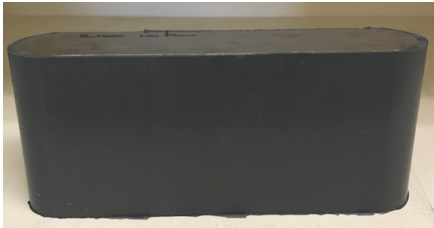
Figure 2.5. Steel plate sample assembly covered in rubber epoxy and ready for testing.
