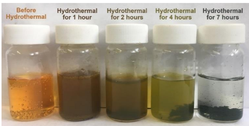
Figure 31. The digital camera photograph of the time-dependent hydrothermal treatment at 200 °C. Different vials from left to right enclose the as-reacted solution/suspension of before hydrothermal, after hydrothermal for 1, 2, 4, and 7 hours.
