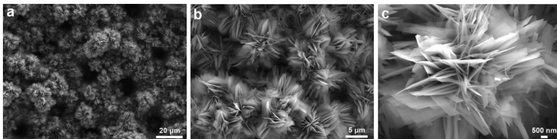
Figure 29. The SEM photographs of unannealed Ni/Porous-Ni/ V_2O_5 nanocomposites at various magnifications. (a) 1500x; (b) 5000x; (c) 15000x.
