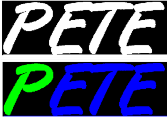
Figure 2.21 The identified connected pixels from binary image: Original image on the top and identified connected objects colored on the bottom
