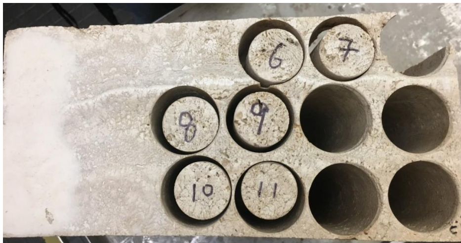
Figure 3.8 Travertine block where the cores are cut from
