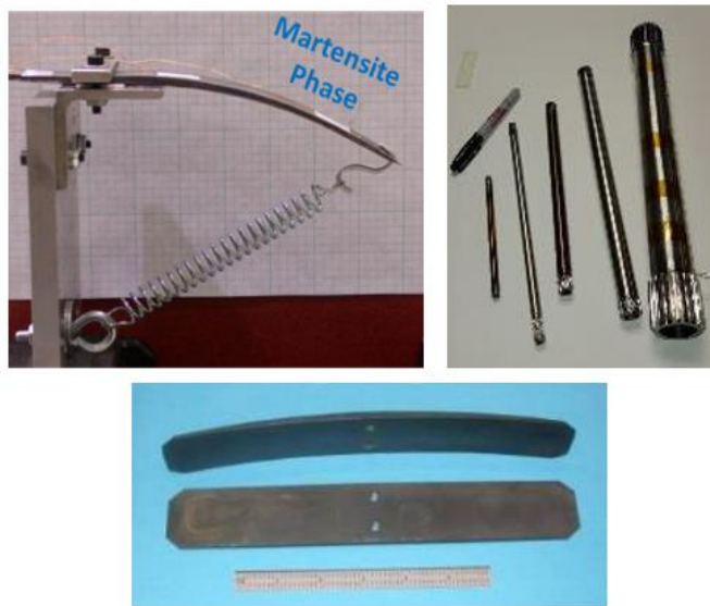
Figure 1.5: Various SMA-based components in the forms of springs, beams and torque tubes that can be used as solid-state actuators.
