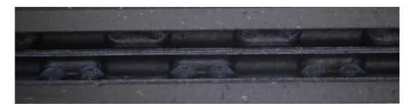
Figure 49: 3D Printed model for TWA with matching elements.
