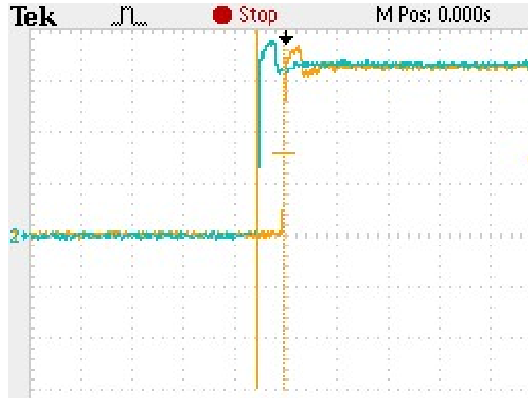
Figure 27: Timing Integrity Evaluation through Comparison of Extracted PPS Signal of Commercial Clock (blue) and GPS Signal (yellow)
