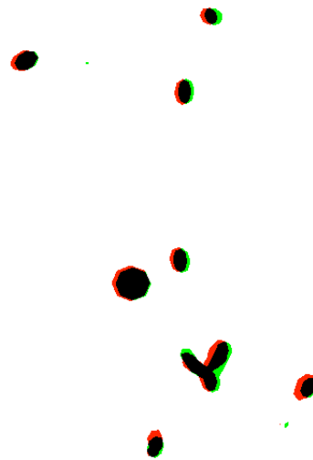
Figure 5.34: Diff image of the same slice acquired from the middle of the 3 \times 3 median filtered ER and the GT. Black pixels are common to both the ER and GT slice; green pixels are in the GT but not the ER; red pixels are in the ER but not the GT.
