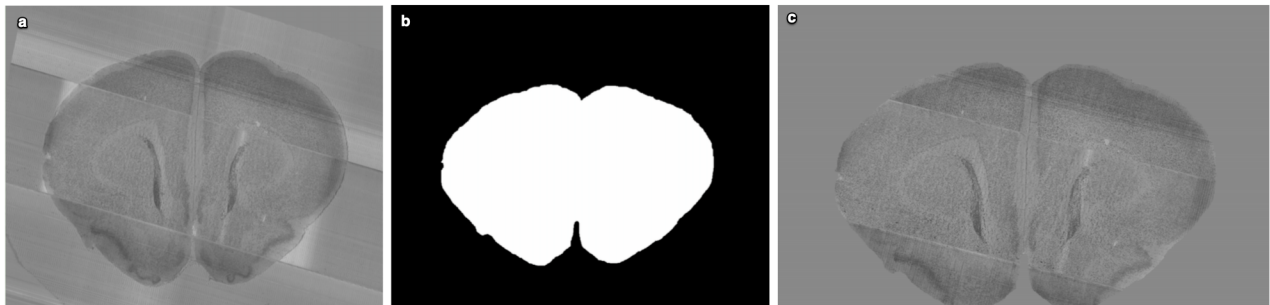
Figure 2.11: Application of freehand brain contour mask to KESM acquired image. (a) Whole-brain image slice with background noise present; (b) freehand brain contour mask generated for (a); (c) application of (b) to (a) to remove noise outside of the brain. Reprinted, with permission, from [6].
