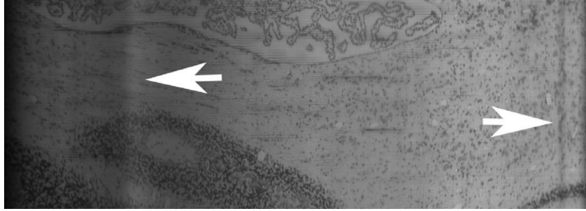
Figure 2.5: Light intensity inconsistencies presenting in KESM imaging. The visible intensity shift along the x-axis is due to knife misalignment; defects in the diamond knife are responsible for the streaks extending along the y-axis (white arrows). Reprinted, with permission, from [3].
