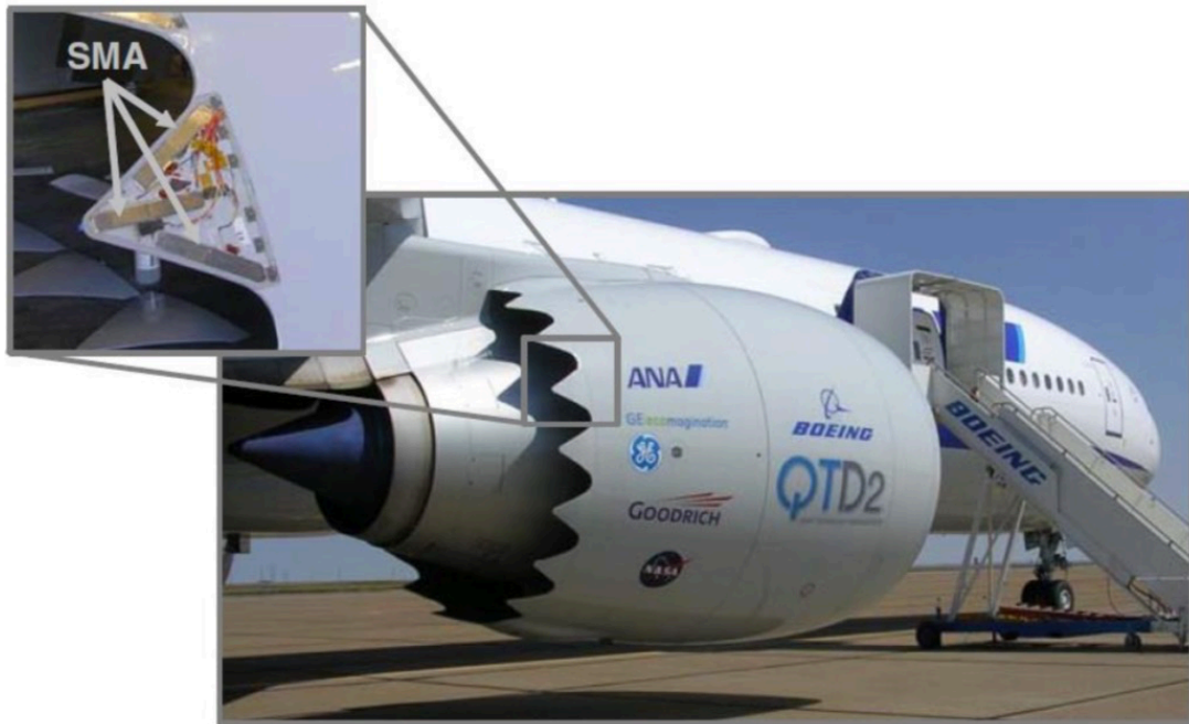
Figure 5 SMA Actuated Chevron on Boeing aircraft reprinted from [10].
