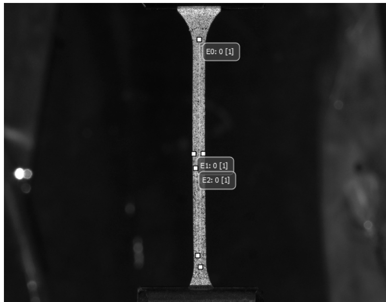
Figure 13 Digital image Correlation speckle pattern used on a flat dogbone for uniaxial tension testing and non-contact extensometer analysis.
