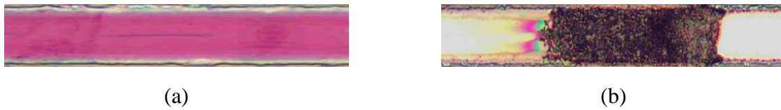
Figure 3.2 Light microscopy images showing the color of a 30 \mu\text{m} wide TiW/Cu/TiW line. (a) before and (b) after line broken from EM stress at J = 1.39 \times 10^6 \text{A/cm}^2 . Reprinted from ref. 50.
