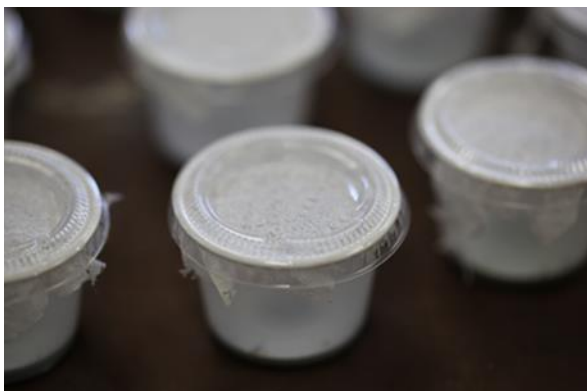
Figure V-1: Bioassay cup depicting single ply tissue paper for ventilation.
