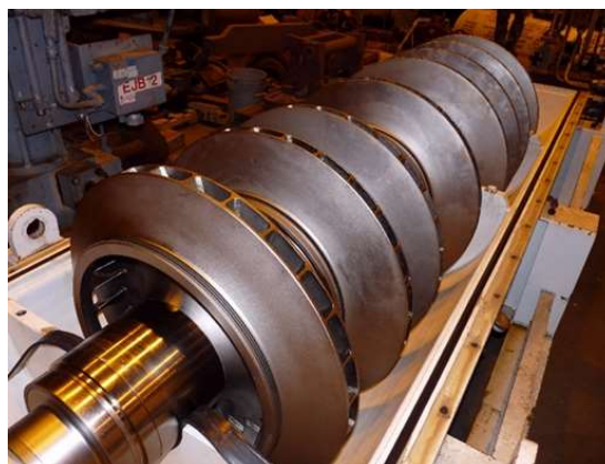
Figure 30: Compressor Rotor with Electroless Nickel Coating
