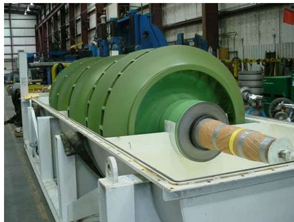
Figure 29: Compressor Rotor with a PTFE Topcoat
