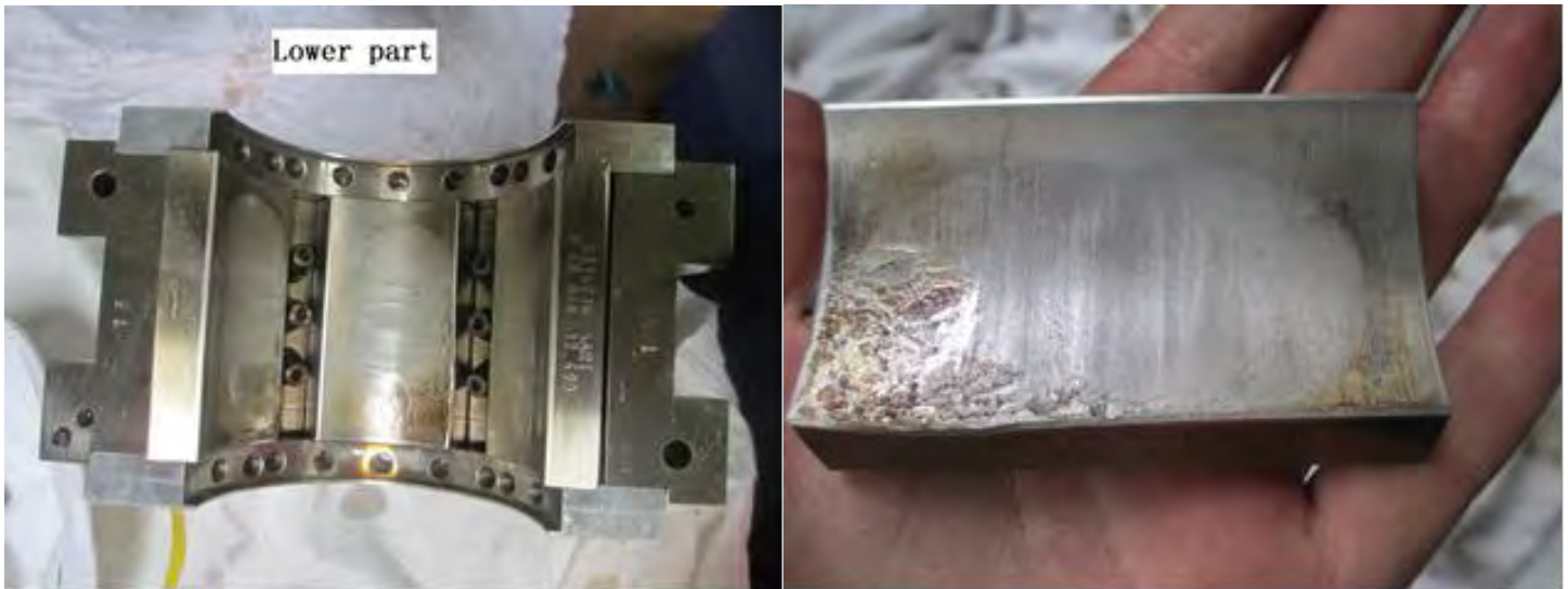
Figure 20: Fourth Stage Bearing Damage for Case Study B
