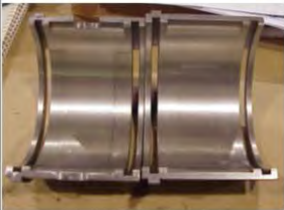
Original Pressure Dam Bearing
