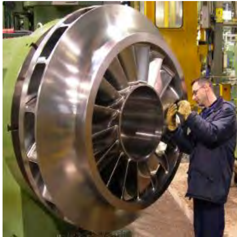
Figure 19. Large 1750 mm (68.9 in.) Diameter Centrifugal Impeller.
