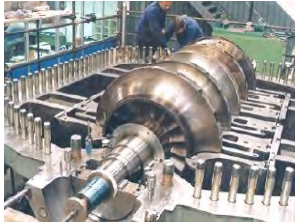
Figure 18. Horizontally Split LNG Centrifugal Compressor.
