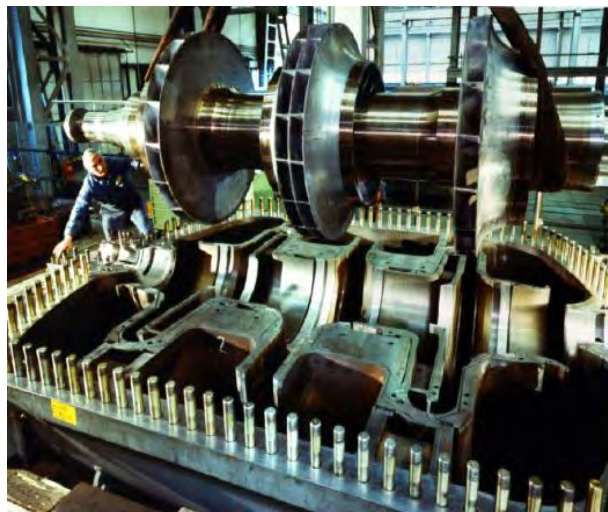
Figure 22. Double Flow Compressor Casing and Rotor.
