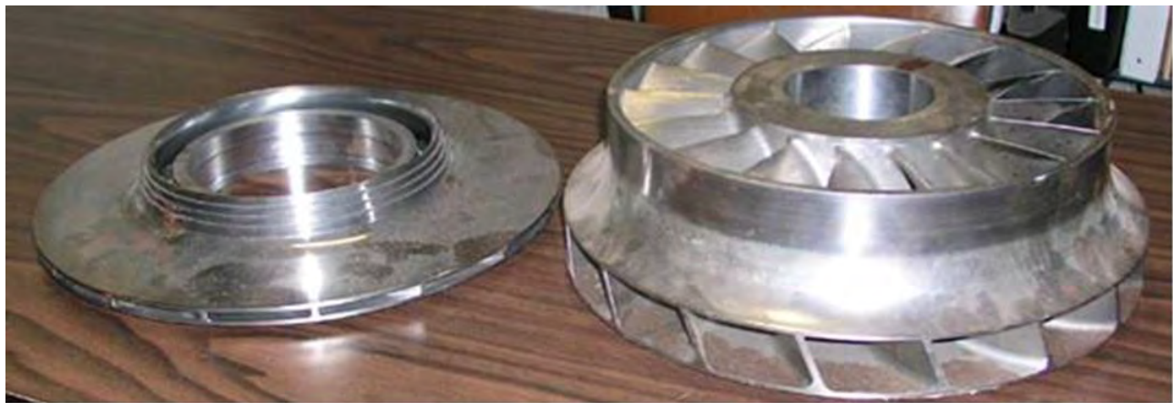
Figure 30. Comparison of Low and High Flow Coefficient Radial Impellers.
