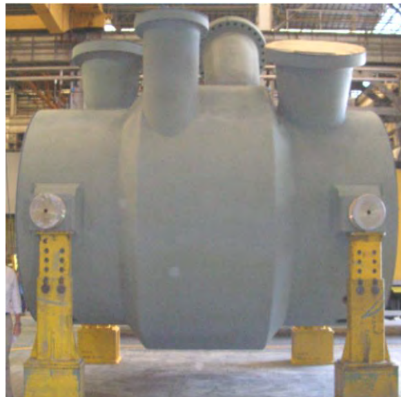
Figure 20. Large Barrel Type LNG Compressor.
