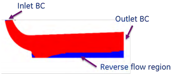
Figure 7. CFD output: cross-section of wheel and diffuser.
