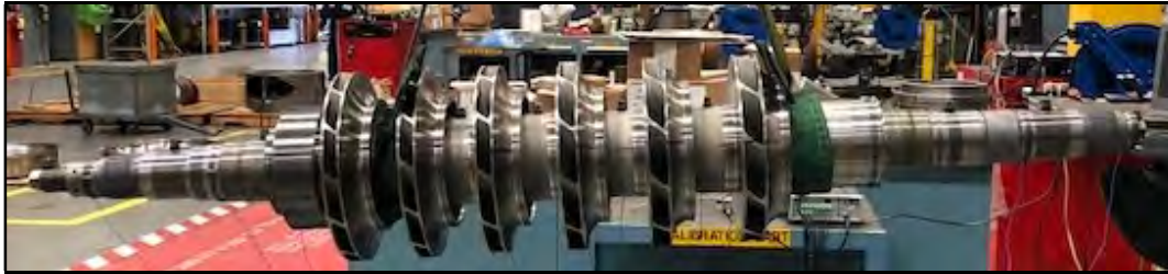
Figure 6: Ring test rotor - suspended in a horizontal position with ten tri-axial accelerometers
