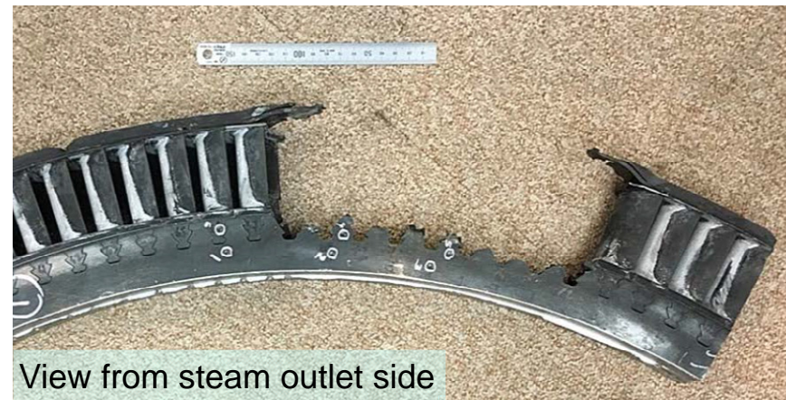
4th stage disk condition (After cut)
