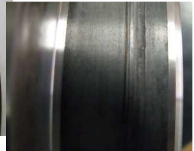
Figure 52: Fretting marks on dynamic
