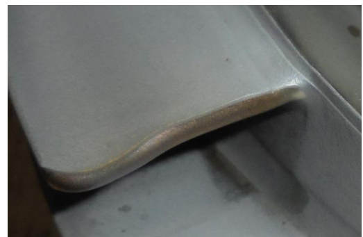
Figure 12. Impeller leading edge after field operation.
