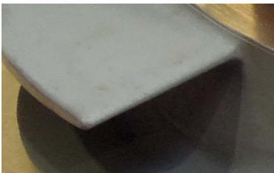
Figure 11. Impeller leading edge prior to installation.
