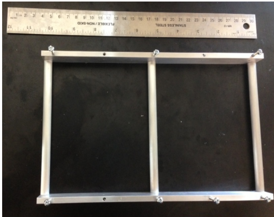
Figure 4: Structure for coating wires. Wires were strung horizontally across this scaffold and secured on either end; coatings were then be wiped on by hand.
