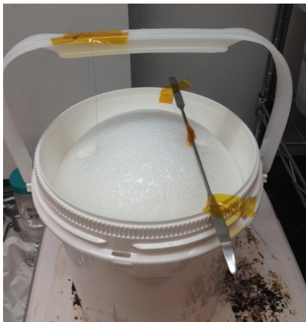
Figure 6: Successful foaming vessel, testing two preliminary ways to secure the wires.
