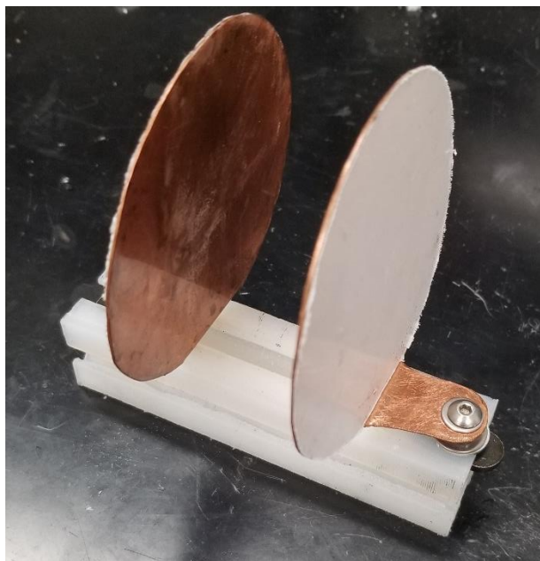
Figure 1. Parallel plate capacitor. Copper disks (diameter 4 in) mounted on a plastic rack.
