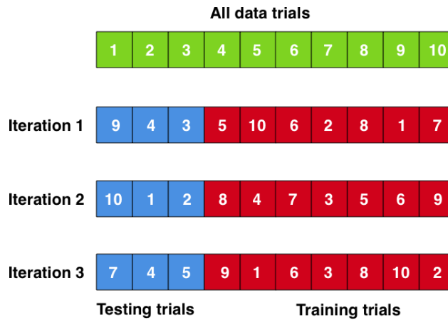
Figure 6. Holdout method in choosing testing and training trials
