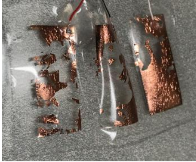
Figure 14. Copper flaking off of the PDMS substrate electrode.
