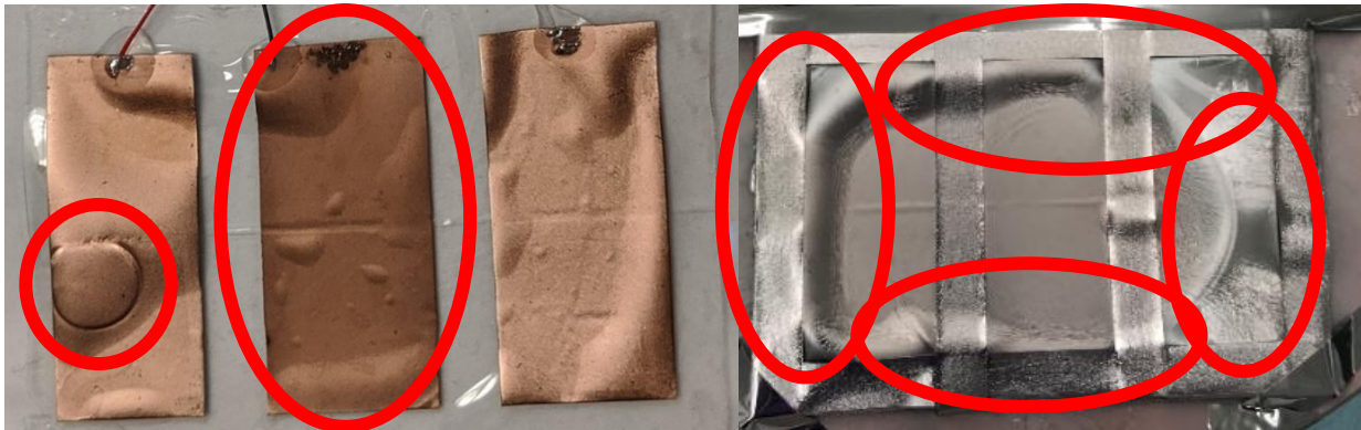
Figure 13. Indications of bubbling occurring in the electrodes prepared in attempt one.
