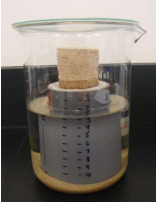
Figure 8. Sand rings used to saturate the soil cores [44]
