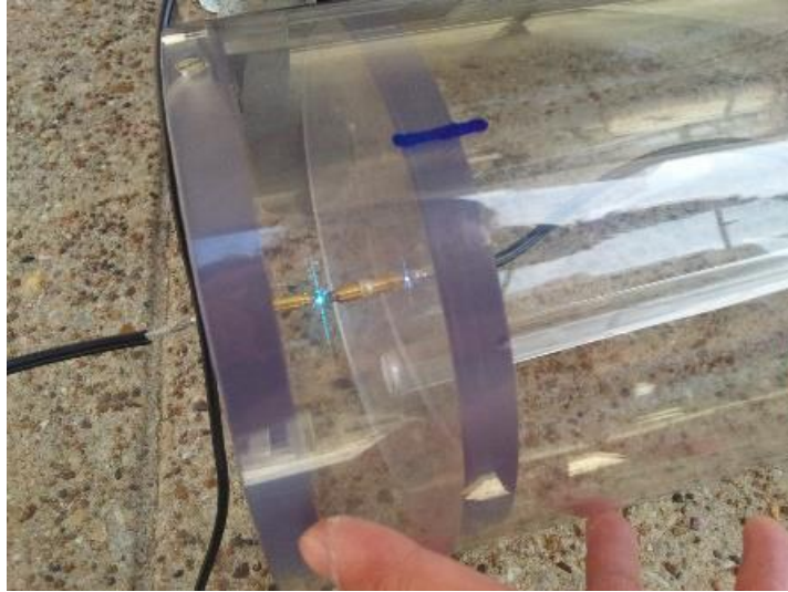
Figure 4. First generation arc fault detector.
