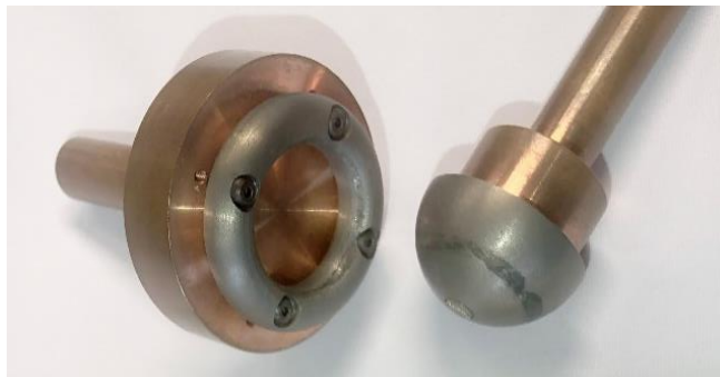
Figure 14. Examples of electrodes with titanium ball and ring geometry.
