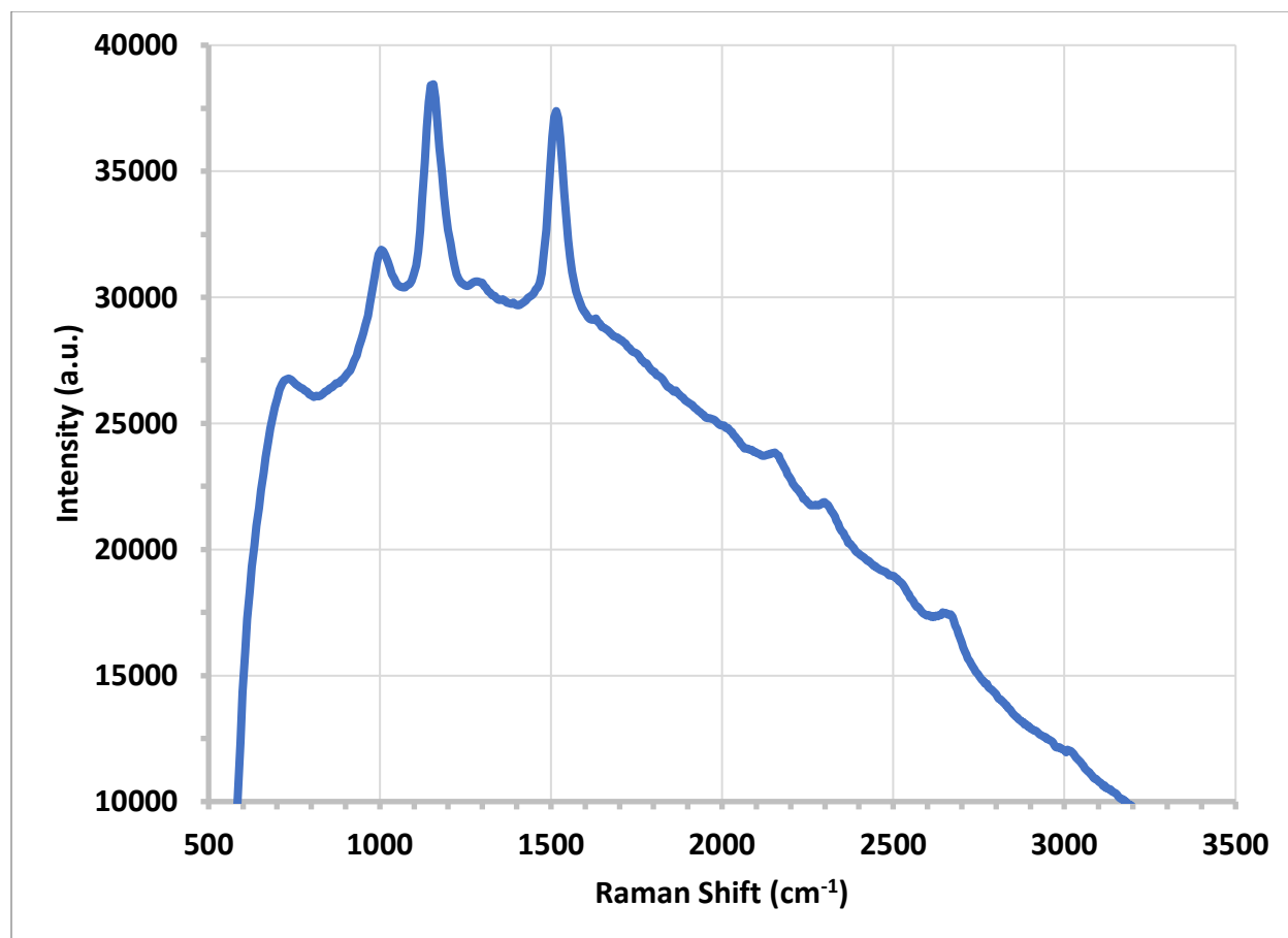
Figure 119: Resonance Raman spectrum of red S. marcescens recorded by portable instrument.
