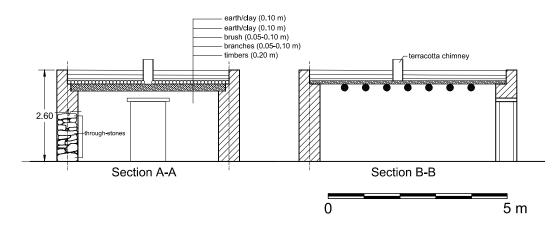
Figure 7: Cross sections of the model house
