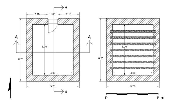
Figure 8: Plan showing walls and door (left) and setting of ceiling beams (right) Alternative plans are also being considered at this stage of design.
