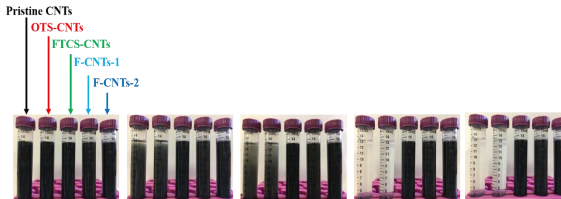
Figure 6. The dispersion images of pristine CNTs, OTS-CNTs, FTCS-CNTs, F-CNTs-1 and F-CNTs-2
