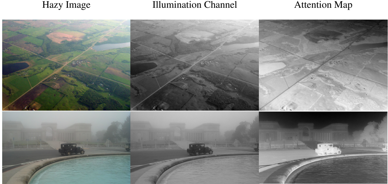
Figure 3.3: Illumination Based Attention Map. The first column represents the input hazy image, the second column uses Eq.3.1 to generate a gray image representing its brightness. The last column is inverse of the illumination channel and it will be used as an attention map input to the generator.
