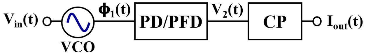
Fig. 45: VCO-based OpAmp block diagram
