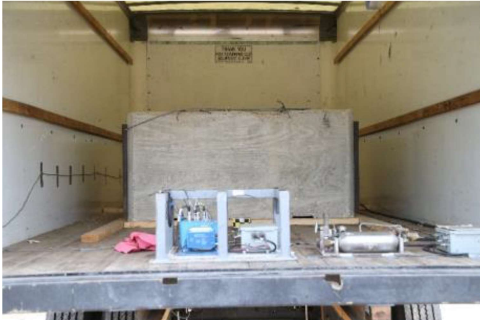
Figure 141 On-Board data acquisition system
