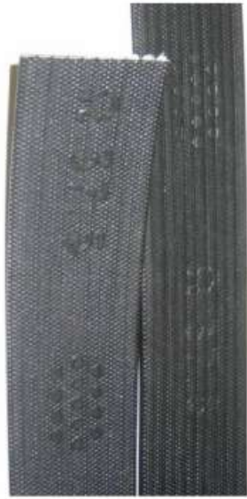
Figure 121 Full strap (left) versus 1/5 of the strap (right) with its edges rolled around a steel tube clamped between the grips.
