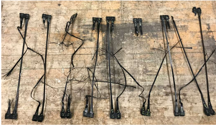
Figure 122 Geogrid specimens after tensile failure
