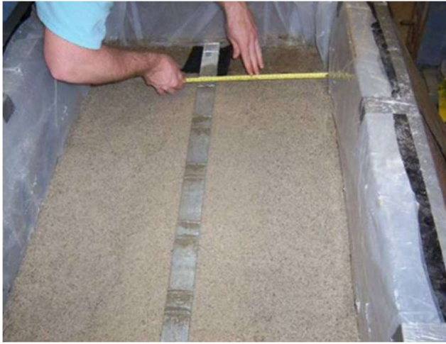
a- Placing the reinforcing strip over sand
