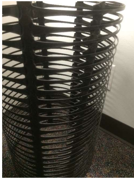
Figure 120 Geogrid roll and clamped sample prior to testing
