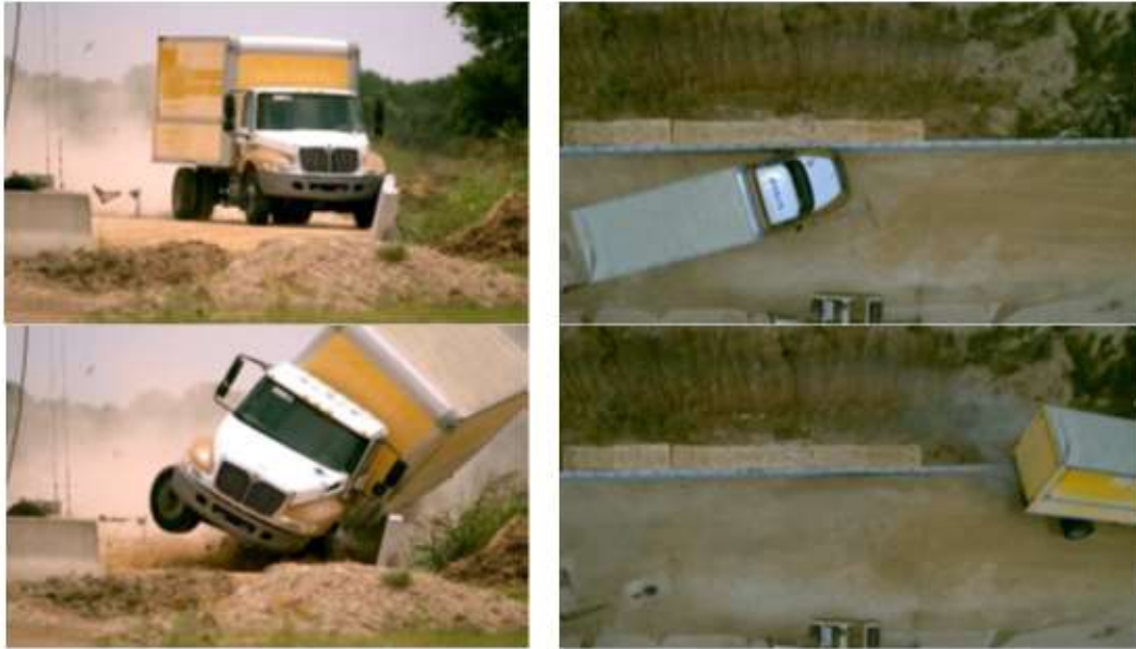
Figure 146 Downstream and overhead photographs of the TL-4 crash test
