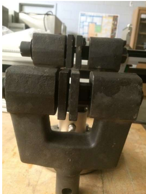
Figure 119 Top and bottom clamps used by tensile testing apparatus
