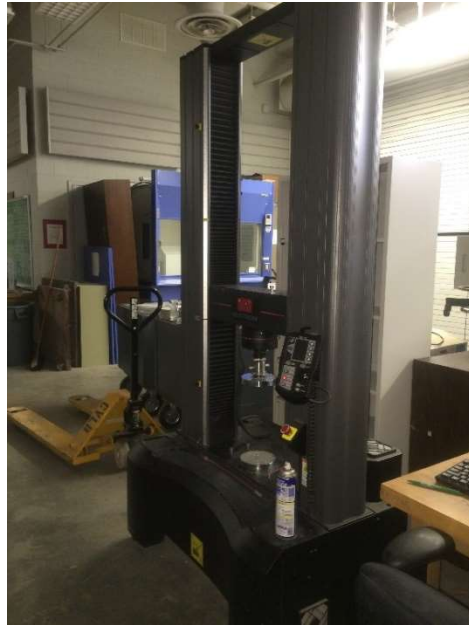
Figure 118 Tensile test device INSTRON 5982
