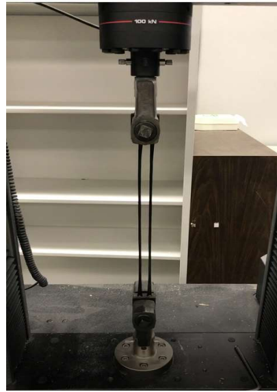
Figure 120 Geogrid roll and clamped sample prior to testing
