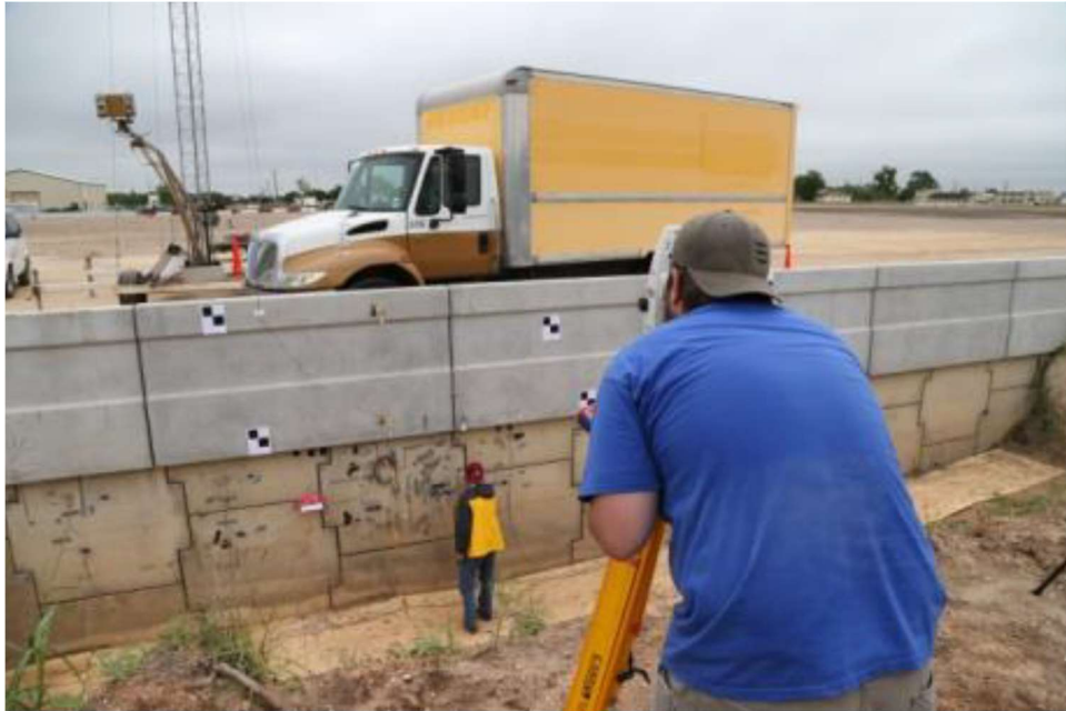
Figure 144 Measurements for permanent displacements before the test
