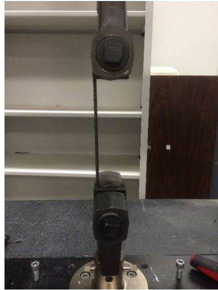
Figure 121 Full strap (left) versus 1/5 of the strap (right) with its edges rolled around a steel tube clamped between the grips.
