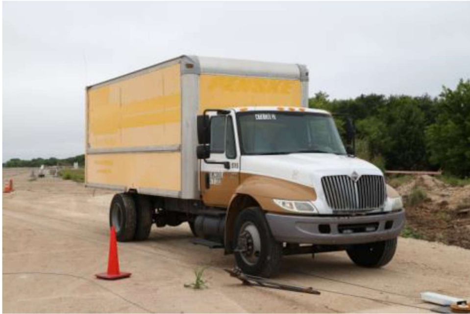
Figure 145 SUT used in the TL-4 crash test
