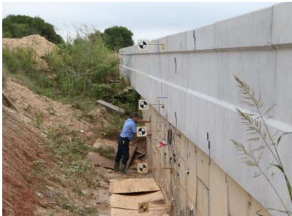
Figure 143 Targets placed on the barrier and panels
