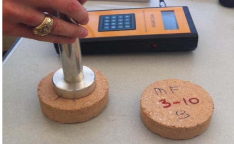
Figure 8.4 Measurement of Dielectric Constant of Base material Using Percometer (Reprinted from Sahin 2014)
