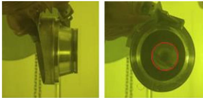
Figure 3. The window welded to the end of the pipe (left) and the beam profile on the window outlined in red (right). Reprinted with permission from [5]
