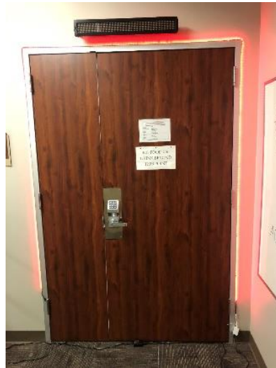
Figure 4: WTAT's LED strip wrapped around the door frame
