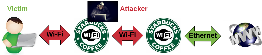
Figure 2.1: Evil Twin AP attack in Wi-Fi infrastructure networks.
