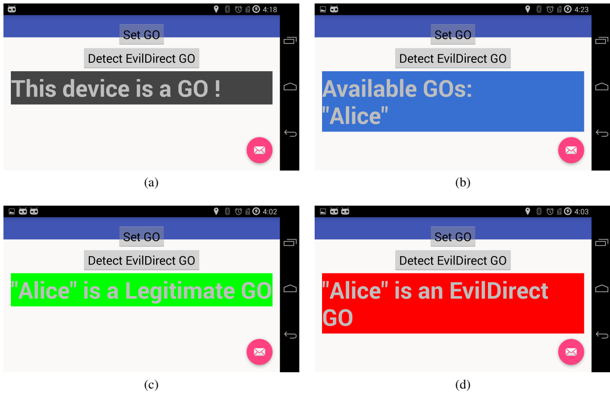
Figure 5.7: “EvilDirectHunter” (a) on GO. (b) on client. (c) Finding legitimate GO. (d) Finding EvilDirect GO. Reprinted with permission from [52].
