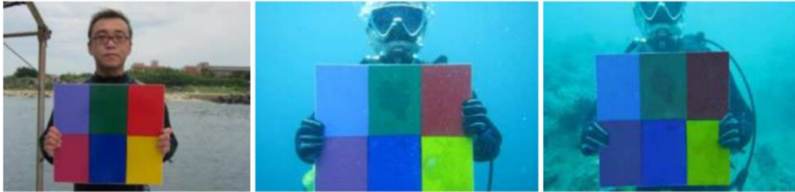
Figure 1.2: Absorption of different colors at different depths in water. From left to right - before diving, diving at a depth of 5 m and diving at a depth of 15 m. Reprinted from [3].
