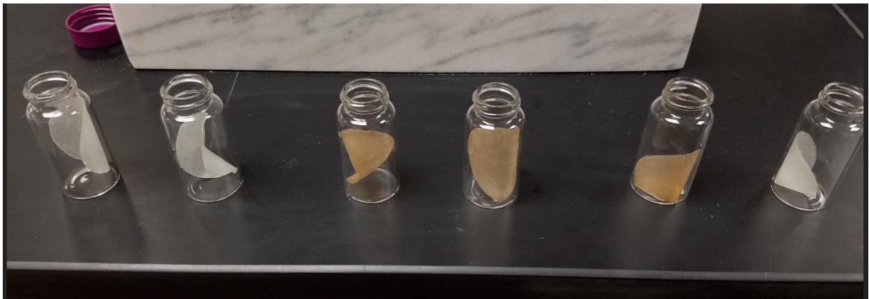
Figure 30: Comparison of filter paper after having new oil and tested oil drained through the filter
