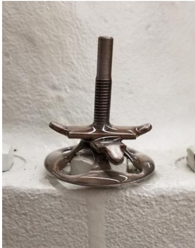
Figure 9: Spider used for oil level setting inside oil bubblers
