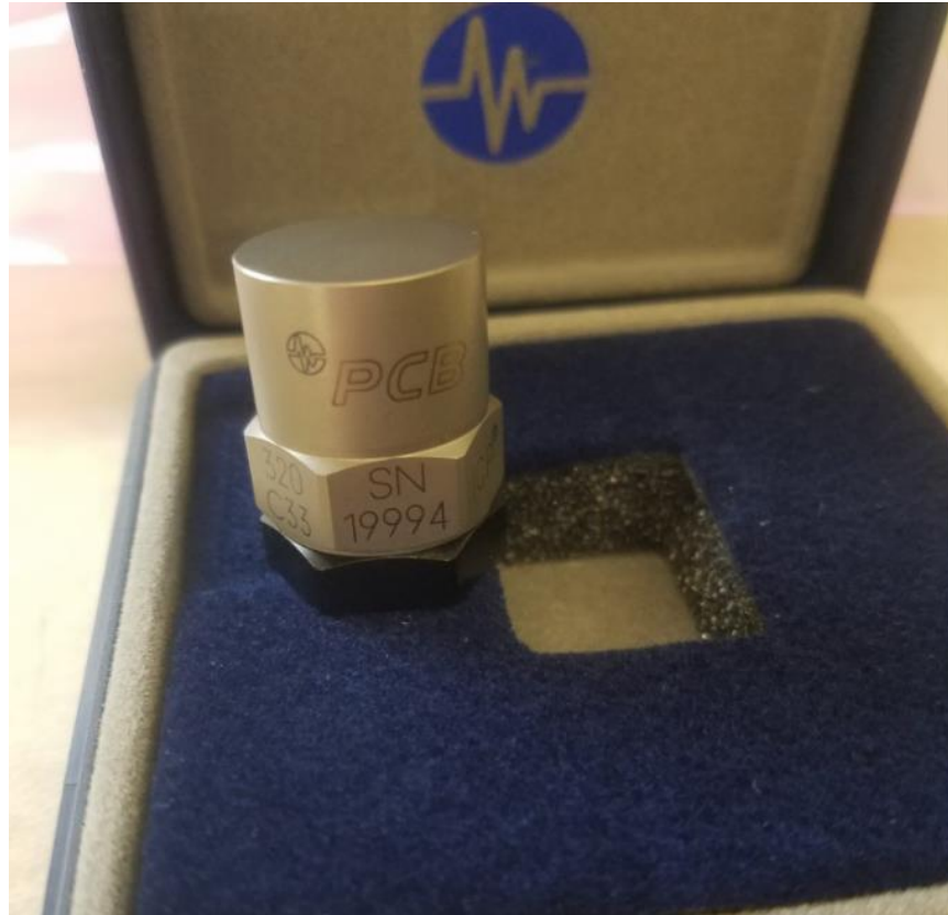
Figure 24: PCB 320C33 accelerometer
