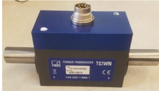
Figure 22: HBM T21WN torque meter
