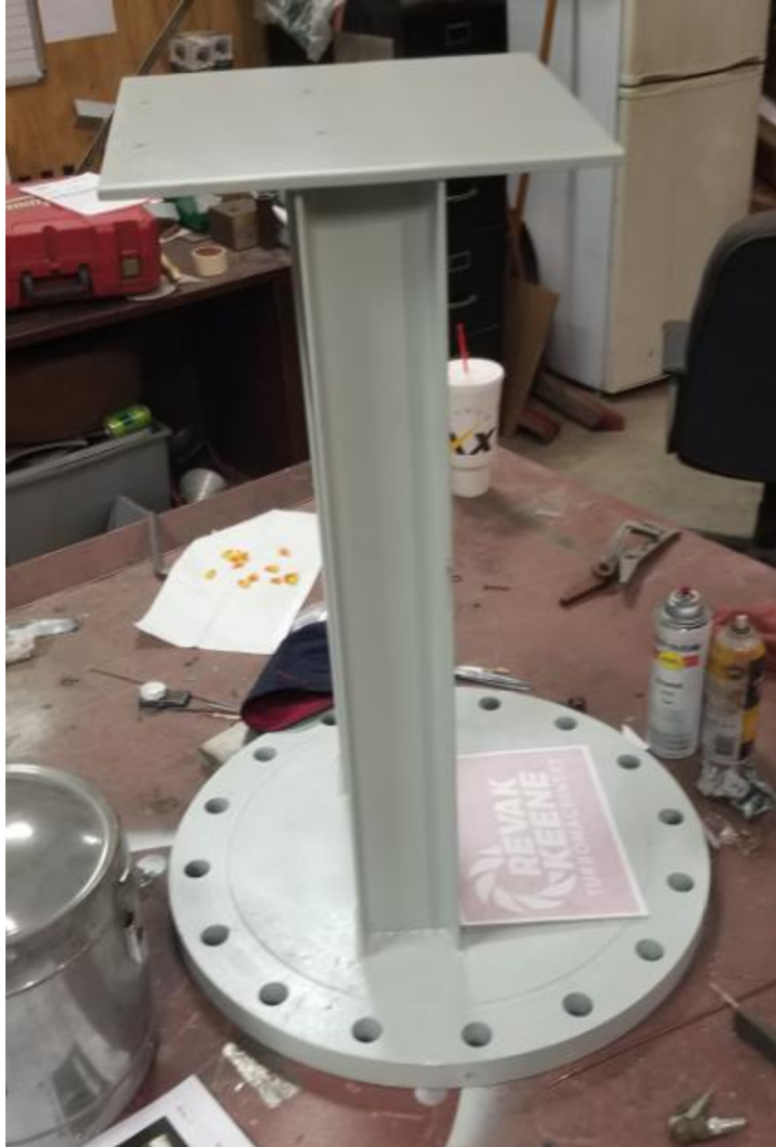
Figure 15: Motor mount for the G series bearing testing
