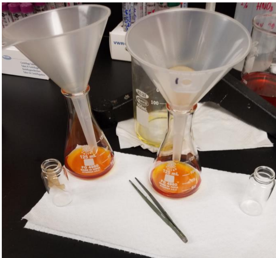
Figure 31: Oil after being through the oil residue test
