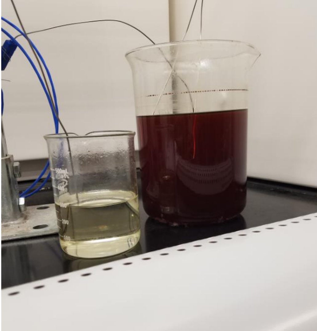
Figure 28: Visual comparison of the tested oil to new oil
