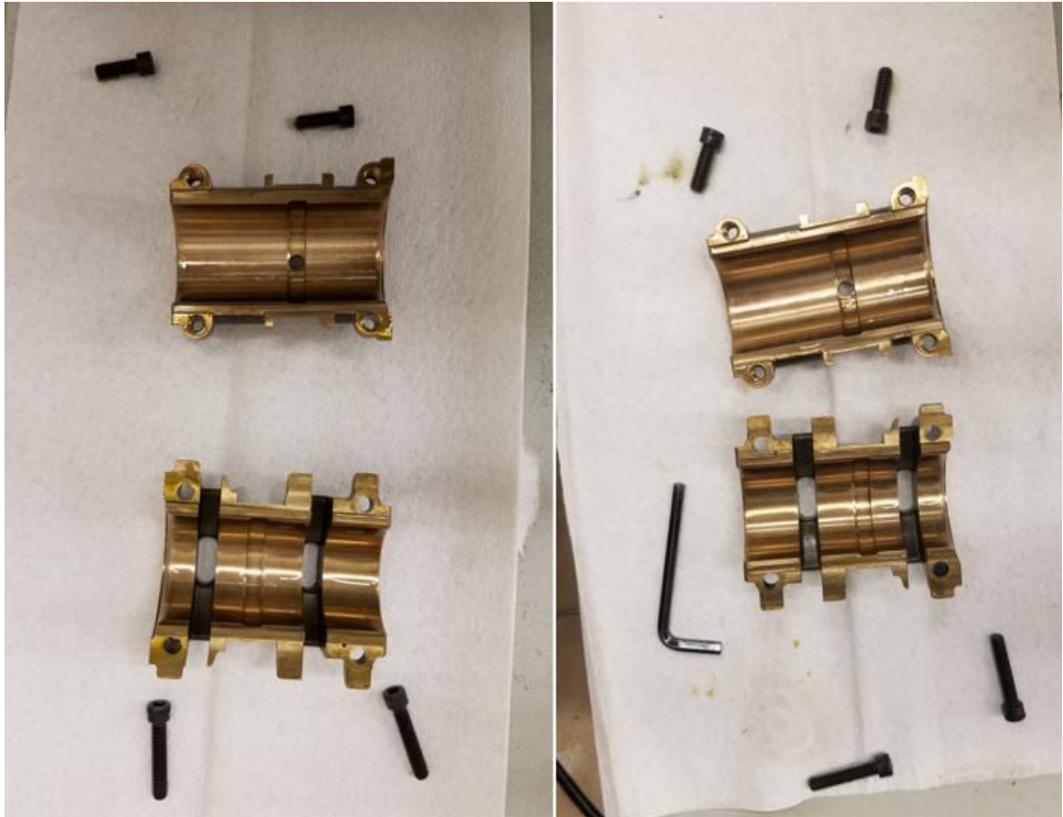
Figure 36: Visual inspection of the bearing before (left) and after (right) the bearing test for the governor end
