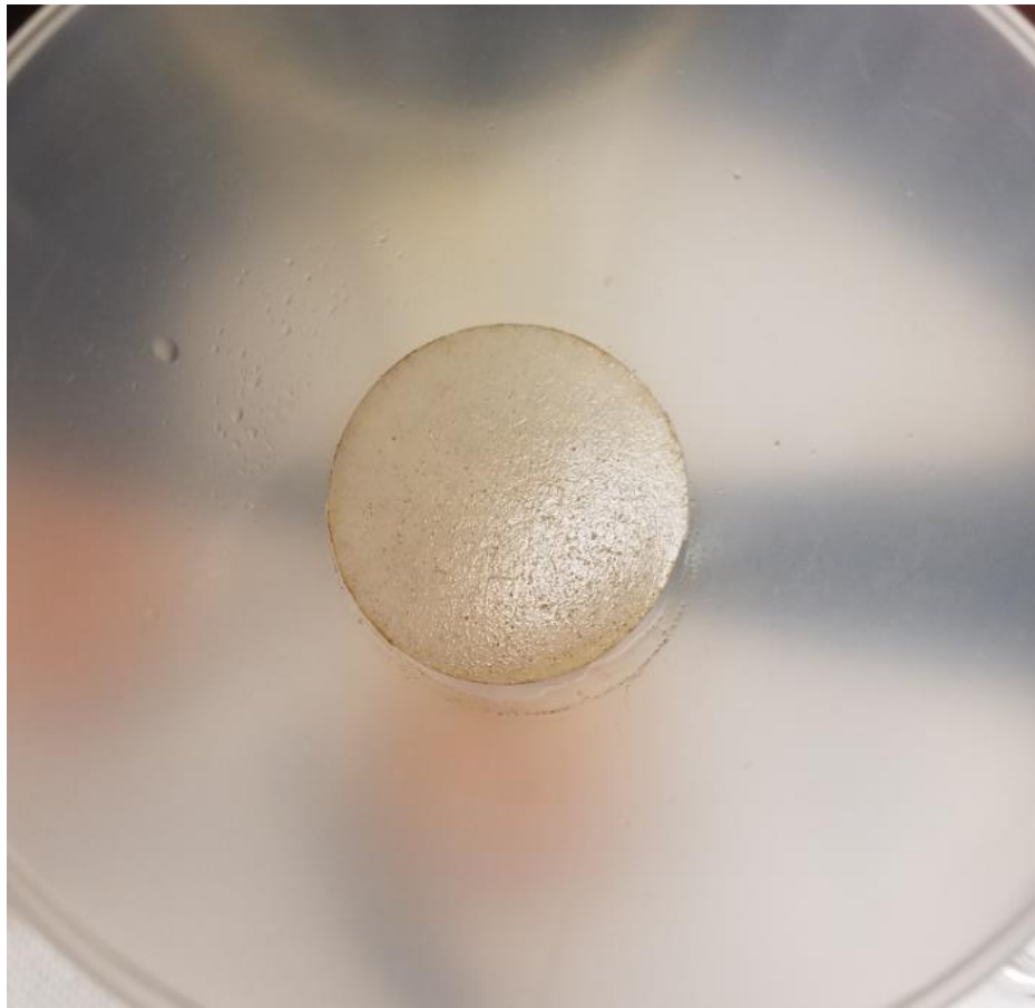
Figure 29: Particulates on filter paper after the oil residue test
