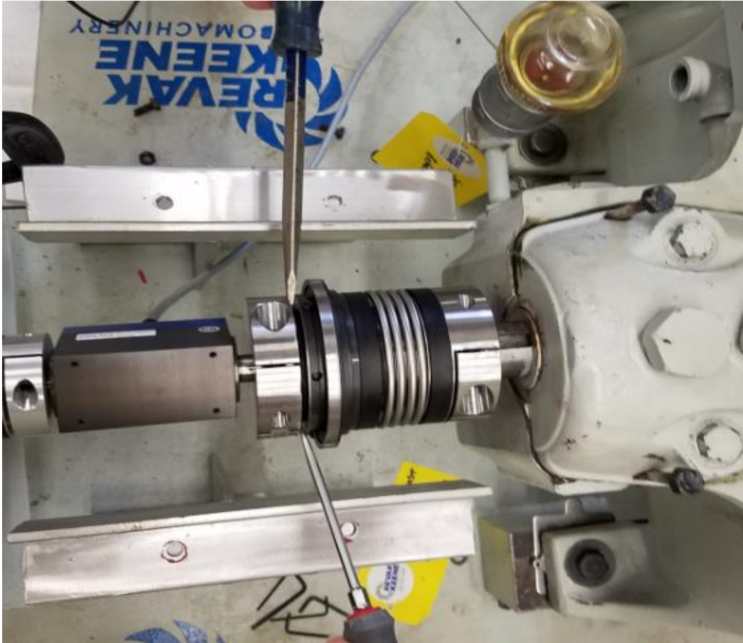
Figure 19: Demonstration of re-engaging the SK2 safety coupling with proper alignment and force points
