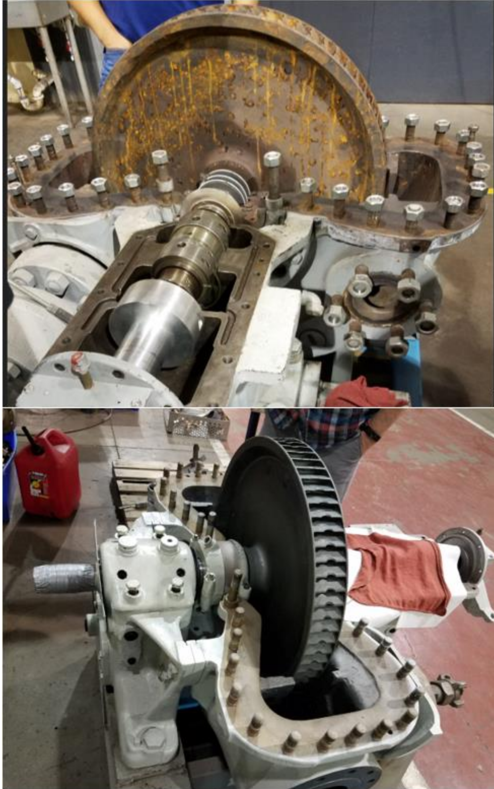
Figure 10: GS-2 Terry turbine from CPS before (top) and after (bottom) refurbishment by Revak-Keene Turbomachinery
