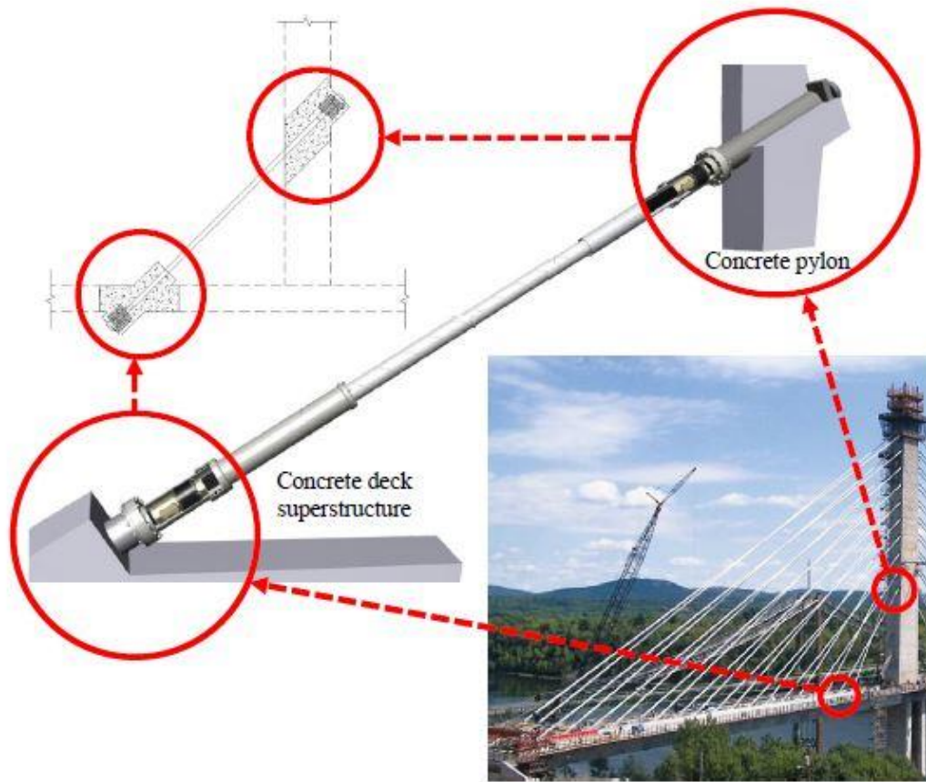
Figure 4-1: Stay Cable End Conditions Mimicked in Mock-Up Specimen (DYWIDAG-Systems International)
