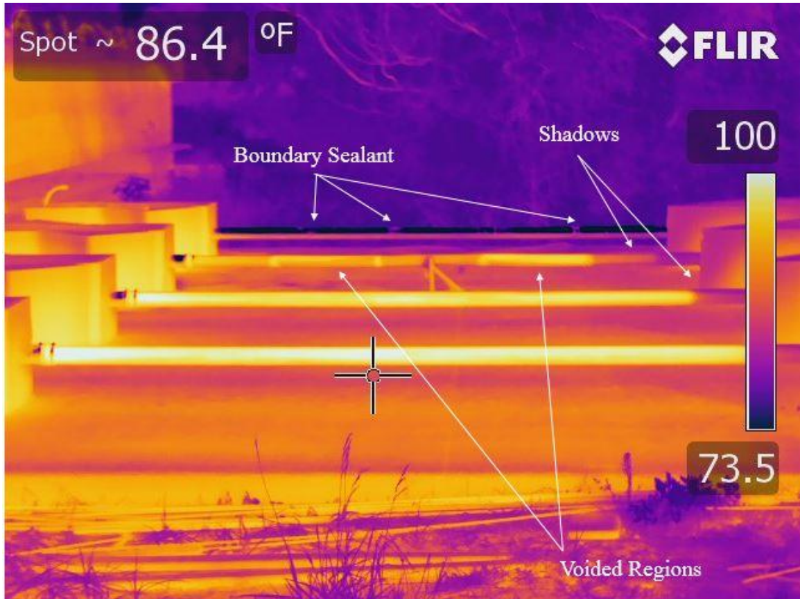
Figure B.3-3: Enlarged Infrared Images of Mock-Up Specimens During Heating Up Period
