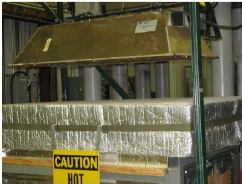
Figure 2-13: IRT Testing Setup with Suspended Heater (Pollock et al., 2008)
