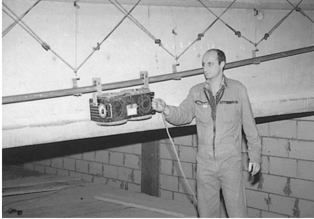
Figure A.2-2. Application of MFL on an external tendon specimen (from Sche et al. 2003).
