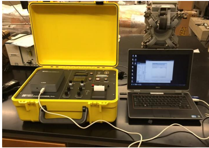
Figure 3-2: CC-04 USB Signal Console Connected to Laptop
