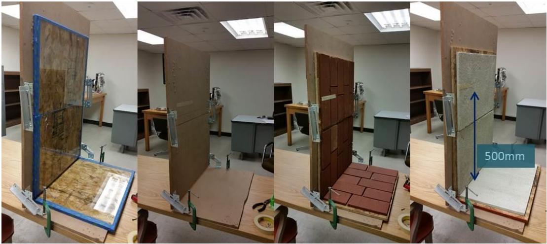
Figure 6: Experimental Setup – Glass, MDF, Brick, and Concrete Climbing Surfaces
