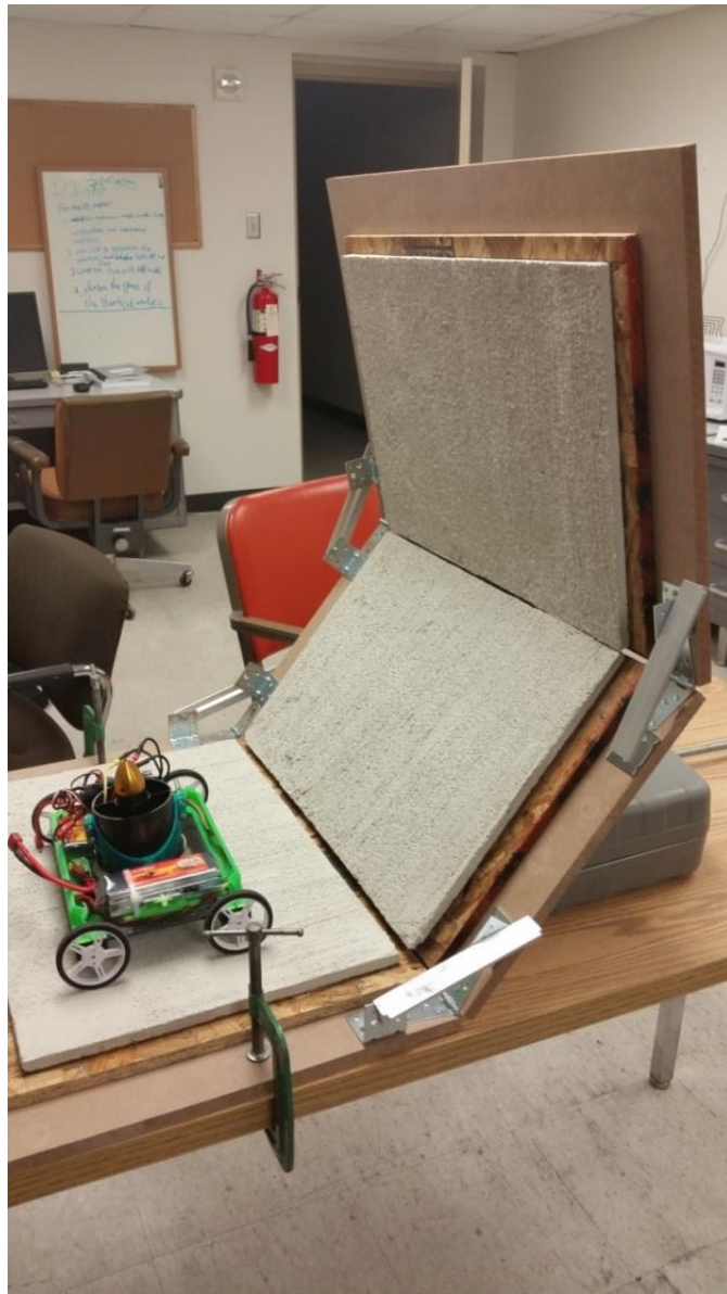
Figure 10: Experiment 3 Actual Setup 130-130 Degree Concrete
