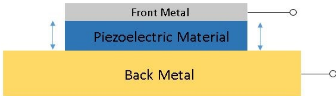
Figure 2: Piezoelectric Transducer Basic Structure
