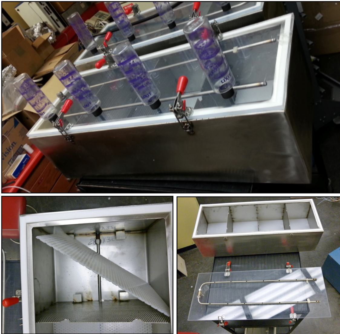
Figure 34. The chambers constructed for the animal exposure experiments.
