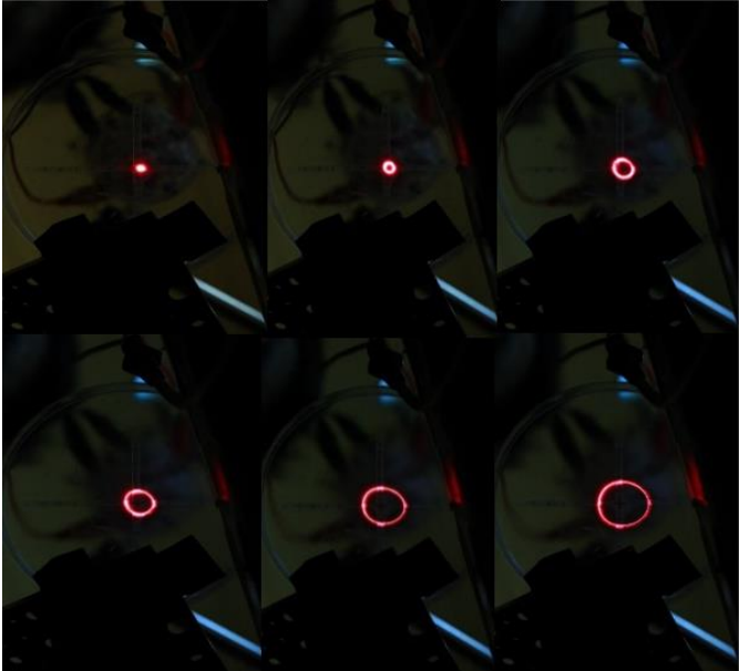
Figure 3.8. Circular scanning pattern with varying scan diameters.
