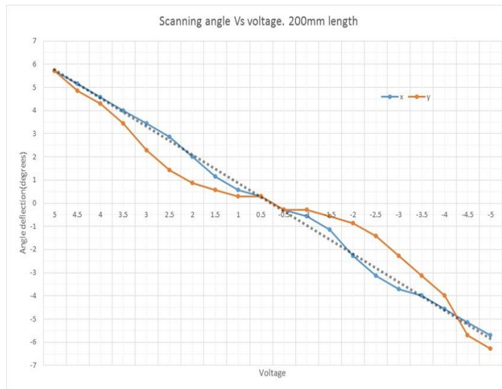
Figure 3.10. Deflection angle characterization data for 200mm long arm. Results are not as linear compared to stiffer arm setup shown previously in figure 3.6.
