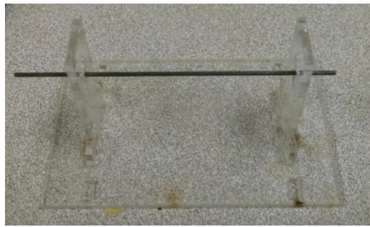
Figure 4.1. Target used for B-scan imaging. The acrylic holder has provision to hold several pencil leads of 0.9mm diameter and varying heights and separations.
