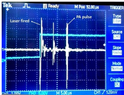
Figure 5.10. Oscilloscope screenshot showing PA pulse received by the ultrasound transducer after the laser has fired and struck the target. At a distance of more than 2cm. Depth information is gleaned from the time taken for US pulse to travel to the transducer once the laser hits the target.
