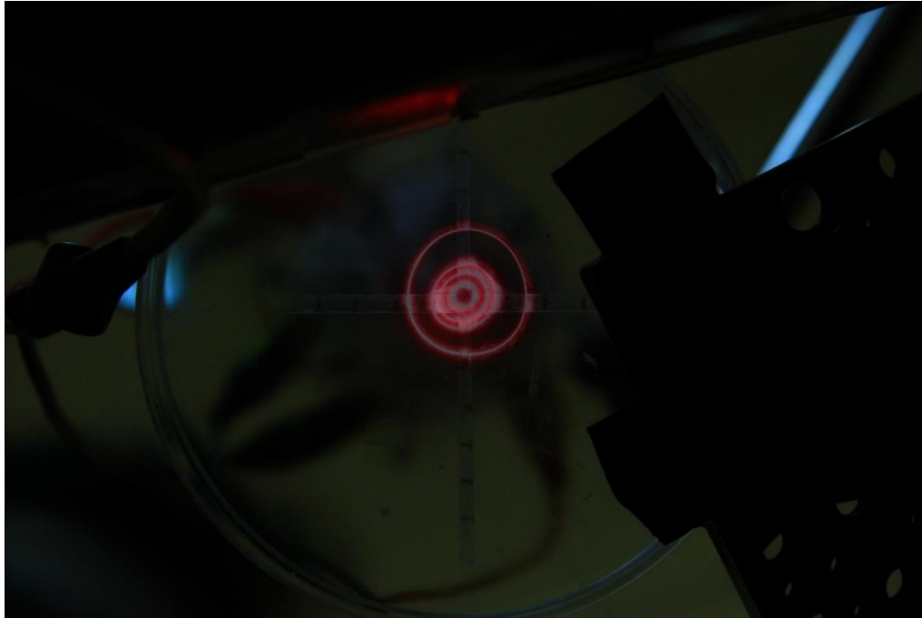
Figure 3.11. Stacked composite image showing distortion of circular pattern as diameter increases.
