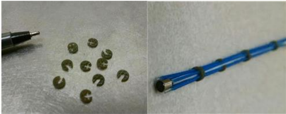
Figure 5.7. 3D printed Spacers (left) and assembled PA probe (right).
