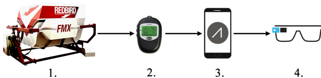
Figure 4.6: Data flow from the Redbird FMX flight simulator (1.) to the Bad Elf GPS device (2.) to an Android smartphone (3.) and finally to Google Glass (4.).
