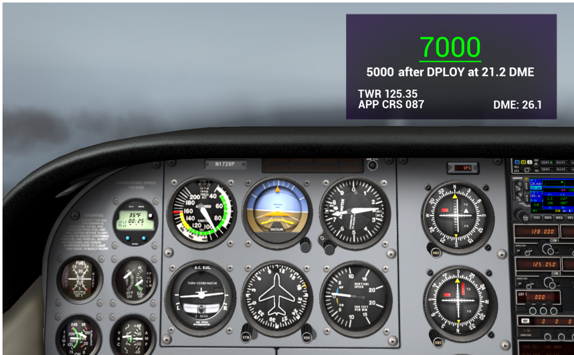
Figure 4.2: A representation (upper right) of what a pilot would see while flying with Google Glass.
