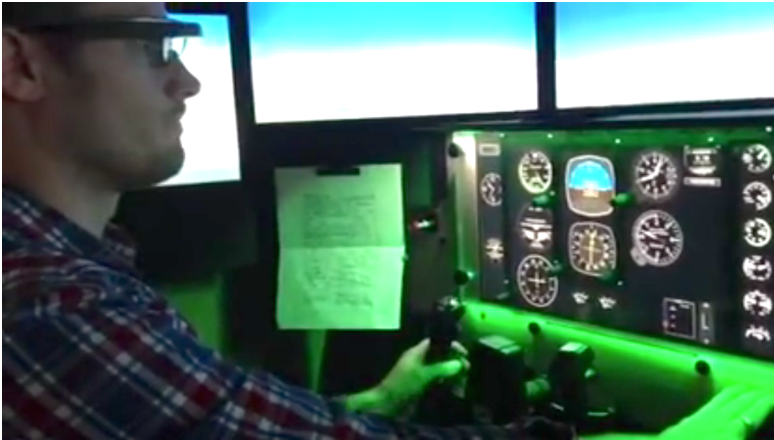
Figure 4.7: In the cockpit of a Redbird FMX flight simulator, the pilot is using Google Glass and the custom-made application.
