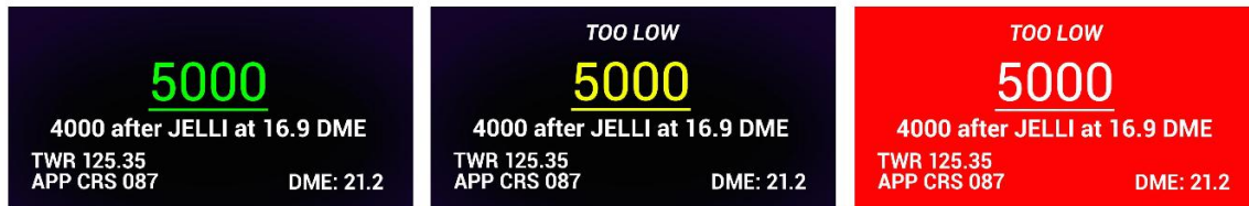
Figure 4.3: Display colors. Green = good; Yellow = warning to stop descending and fix altitude; Red = ascend immediately to avoid danger.
