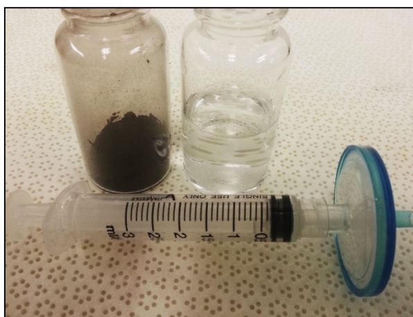
Figure 67. Crushed rock and triple filtered solution for zeta potential determination
