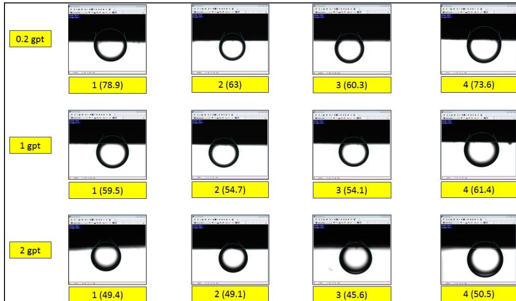
Figure 44. Contact angle results for S-1 with surfactant N1
