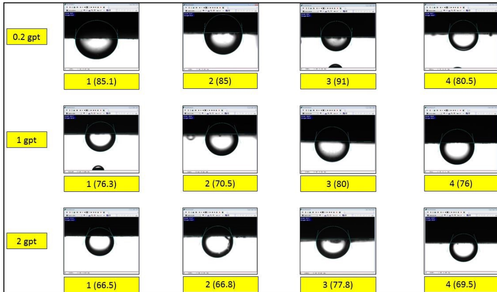
Figure 42. Contact angle results for SW-1 with surfactant C1
