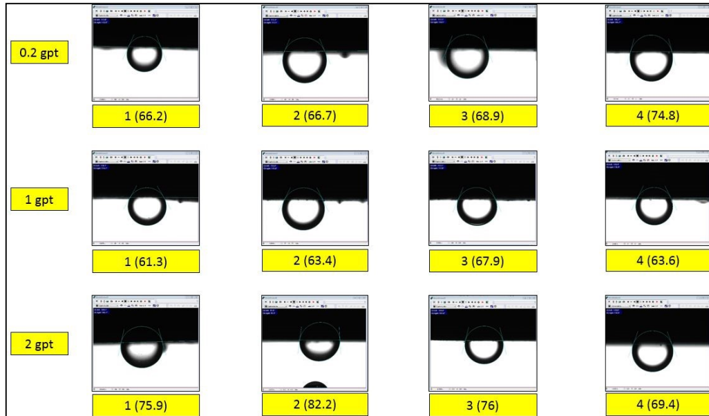
Figure 45. Contact angle results for S-1 with surfactant C1
