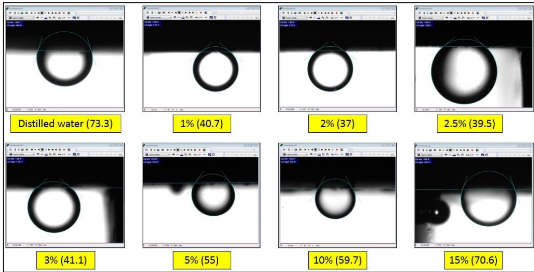
Figure 32. Contact angle results for S1-3 with NaCl brine
