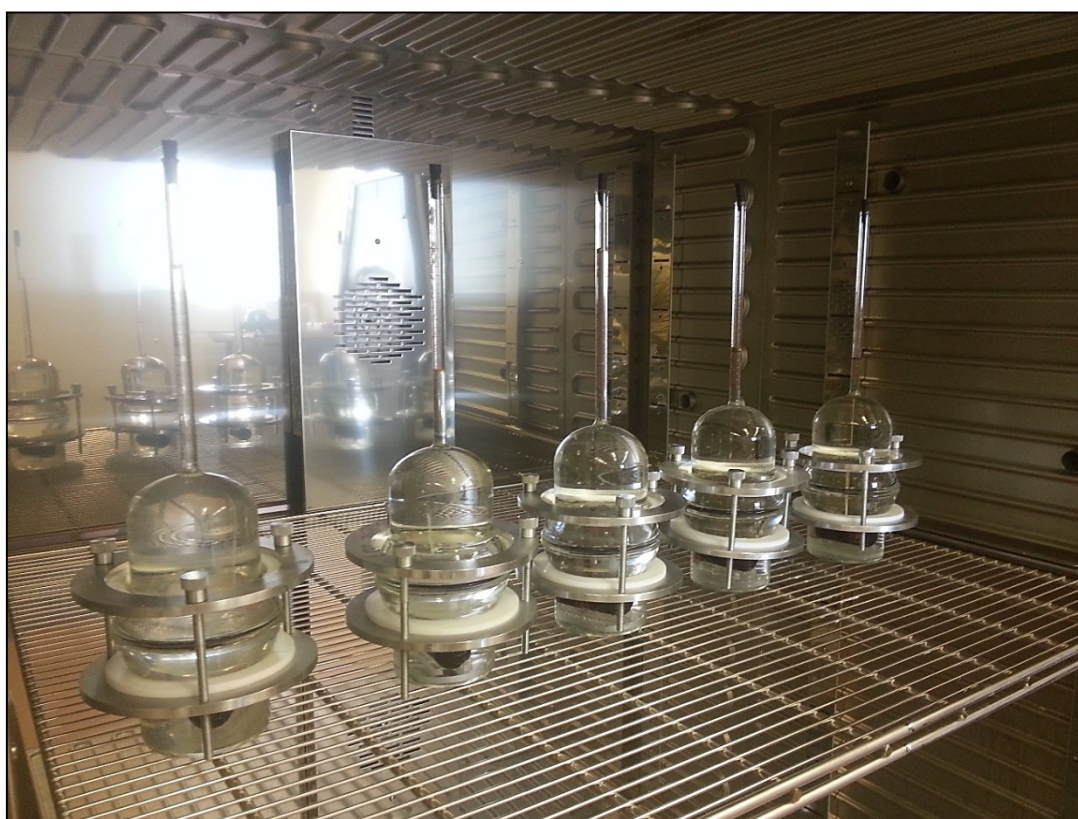
Figure 77. Amott cells placed in the oven at a fixed temperature of 180°F
