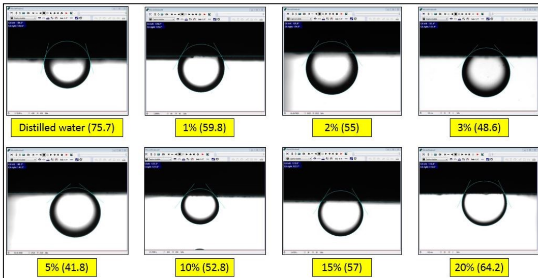
Figure 31. Contact angle results for S1-1 with CaCl 2 brine
