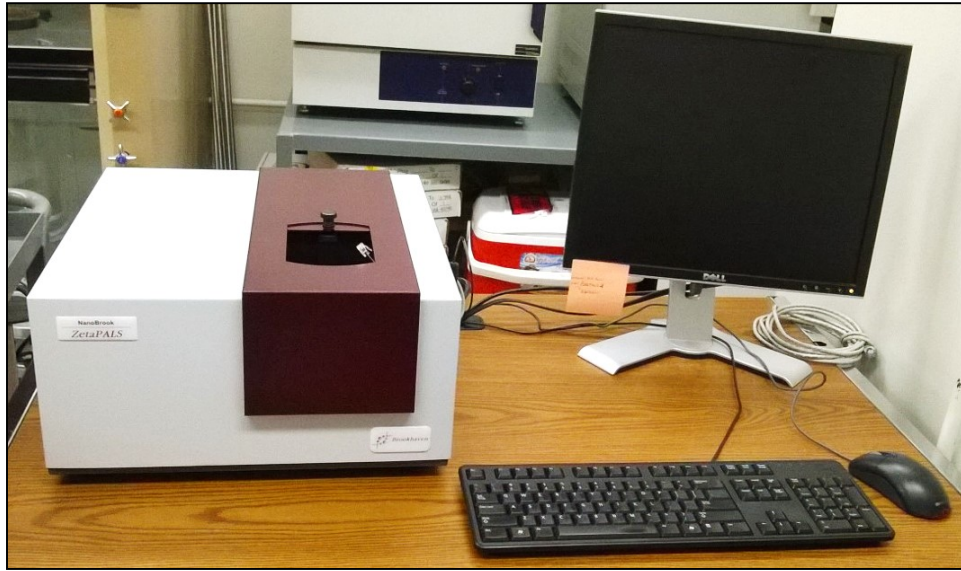
Figure 64. NanoBrook ZetaPALS machine for measuring zeta potential
