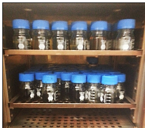
Figure 19. Core samples being aged in the Yamato DX 400 oven at 180°F
