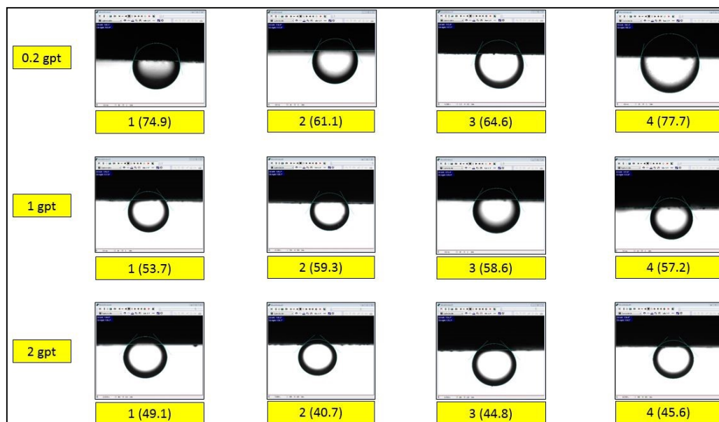
Figure 43. Contact angle results for S-1 with surfactant A1
