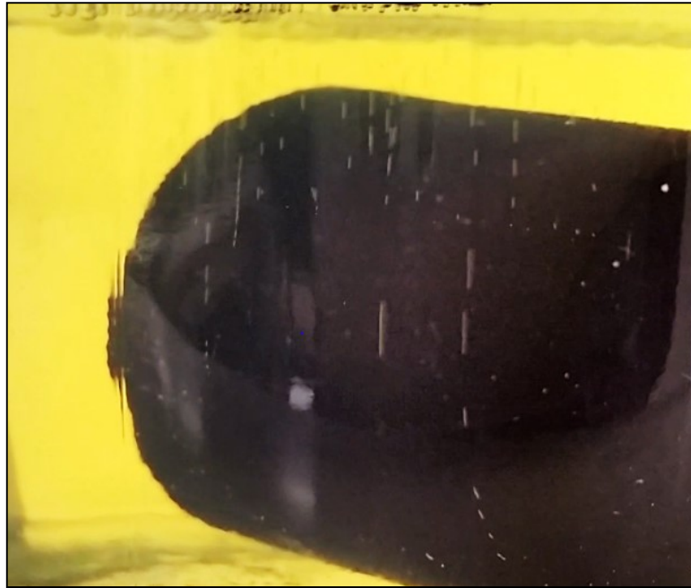
Figure 79. Release of air/gas bubbles during aging process
