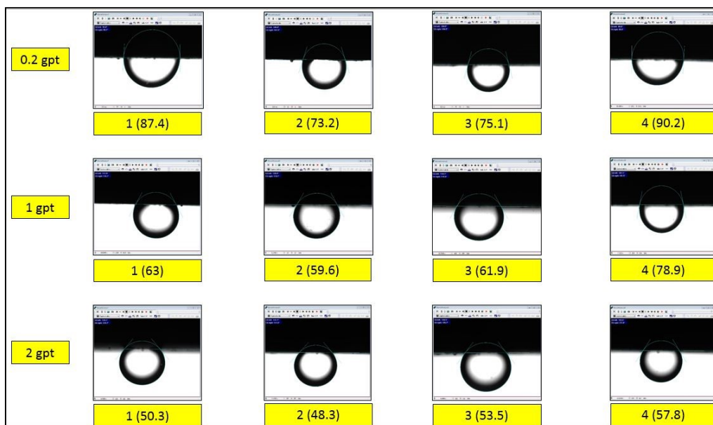
Figure 41. Contact angle results for SW-1 with surfactant N1
