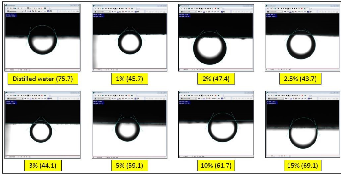
Figure 30. Contact angle results for S1-1 with NaCl brine
