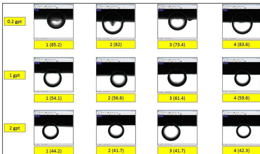
Figure 40. Contact angle results for SW-1 with surfactant A1
