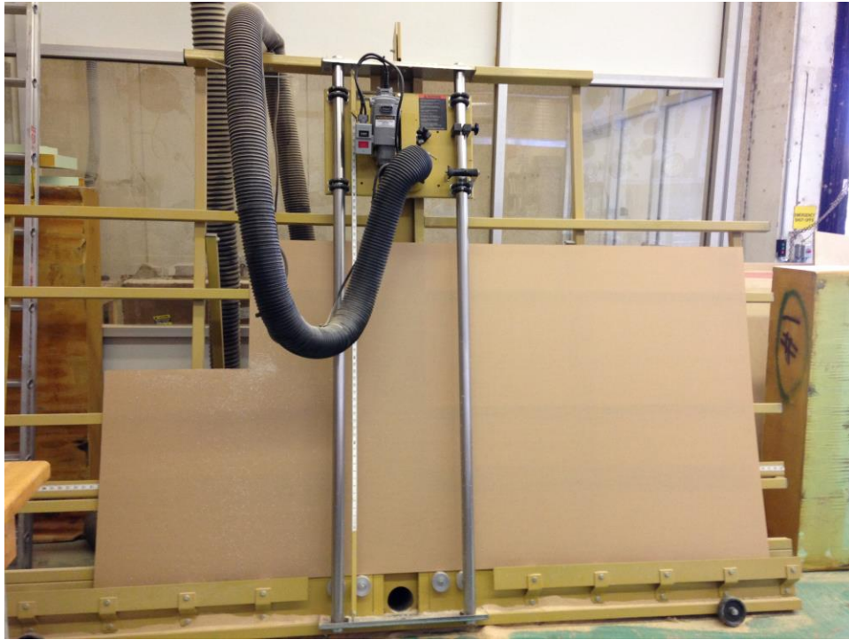
Figure 10. Panel saw used to cut MDF and thermal insulation
