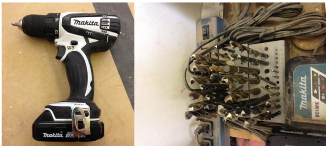
Figure 13. Drill with drill bits to bore holes or drive screws
