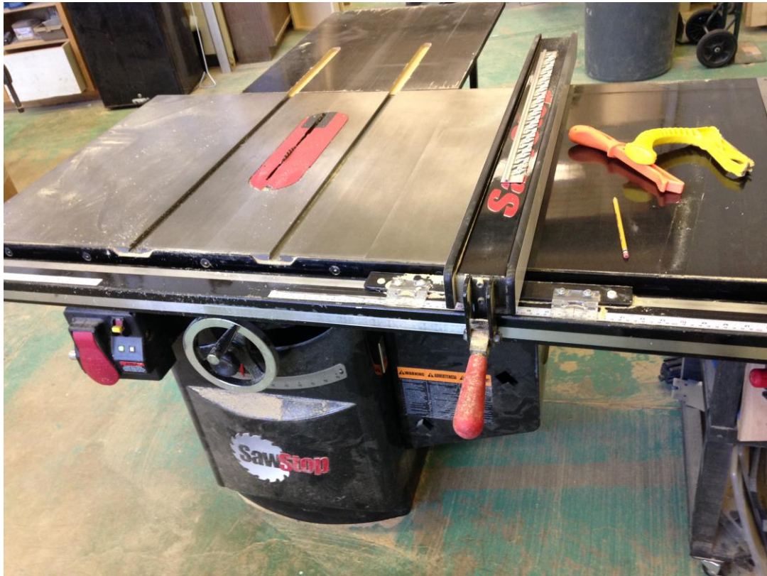
Figure 11. Table saw used to cut MDF, specimens and thermal insulation
