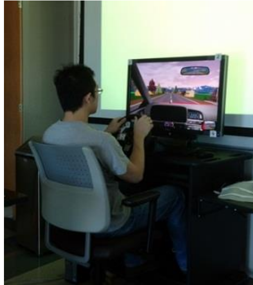
Figure 30. Driving simulation scenario, with the ambient-visual display projected to the background screen behind the monitor.
